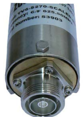
7/16" DIN female at base of antenna
