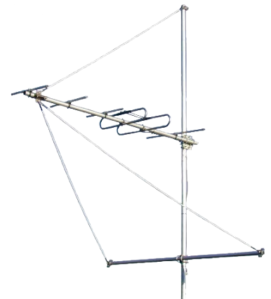
Y206-1722 with tension strut and double compression strut, suitable for extreme wind locations or alpine regions with snow/ice
