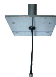
N-type female termination fitted to external RG142B/U coaxial cable
