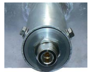
N-type female in base of launcher assembly extends to the rear of the dish for easy connection.
