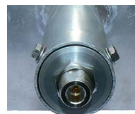
N-type female in base of launcher assembly extends to the rear of the dish for easy connection.
